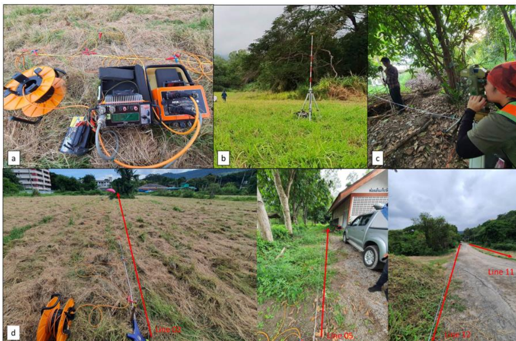
Fig. 4 (a) Electrical resistivity survey instruments, (b) real time kinematic GPS, (c) auto level with electronic distance measurement for survey coordinates, and (d) some of survey lines.
