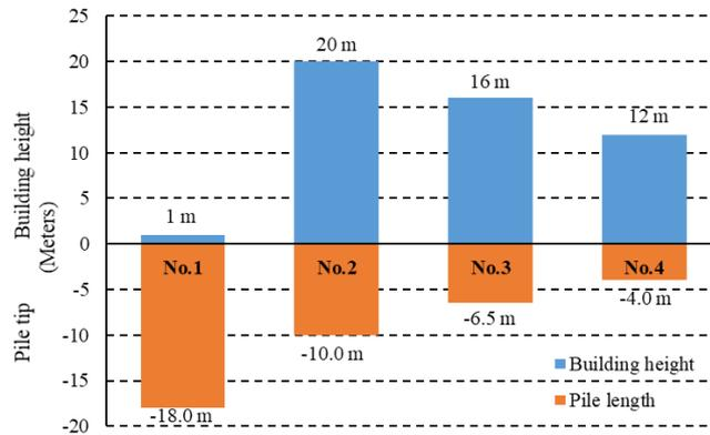
Fig. 4 Heights and depths of four concrete structures tested by PSPT
