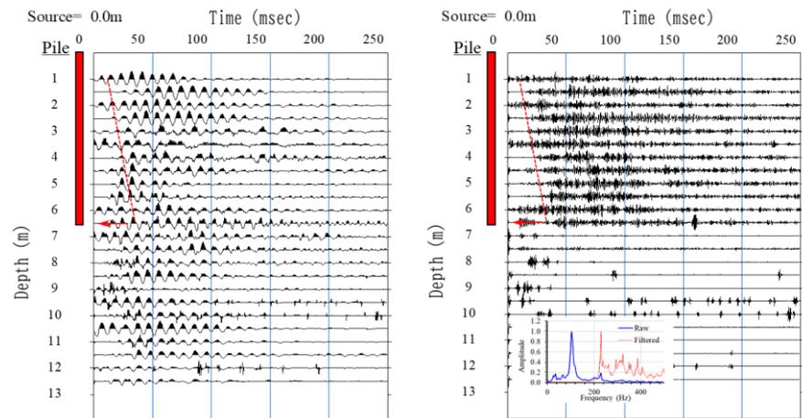
Fig. 7 PSPT result of building No.3: raw data (left) and filtered data (right)
