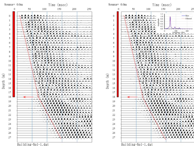
**Fig. 5** PSPT result of building No.1: raw data (left) and filtered data (right)
