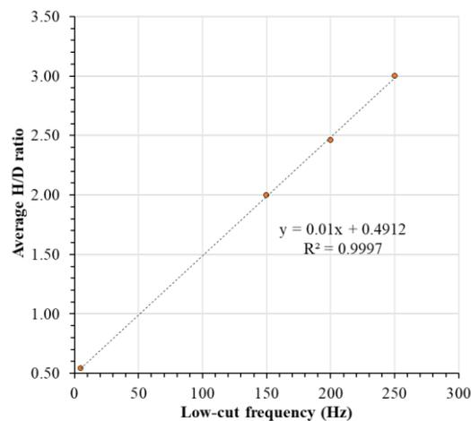
**Fig. 10** Relationship between the H/D ratio and the optimized low-cut frequency
