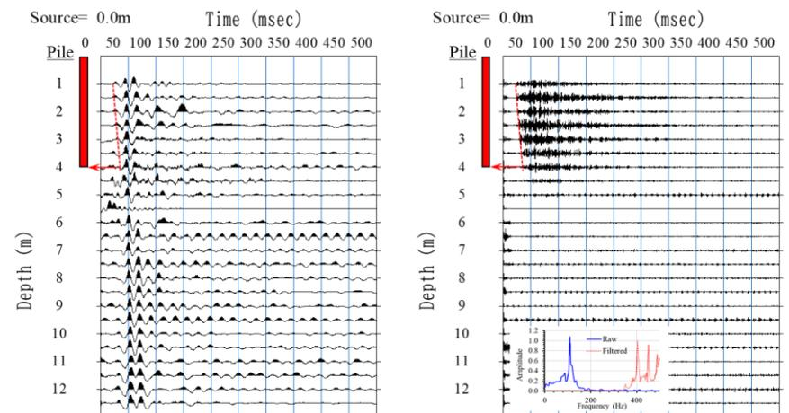
Fig. 8 PSPT result of building No.4: raw data (left) and filtered data (right)
