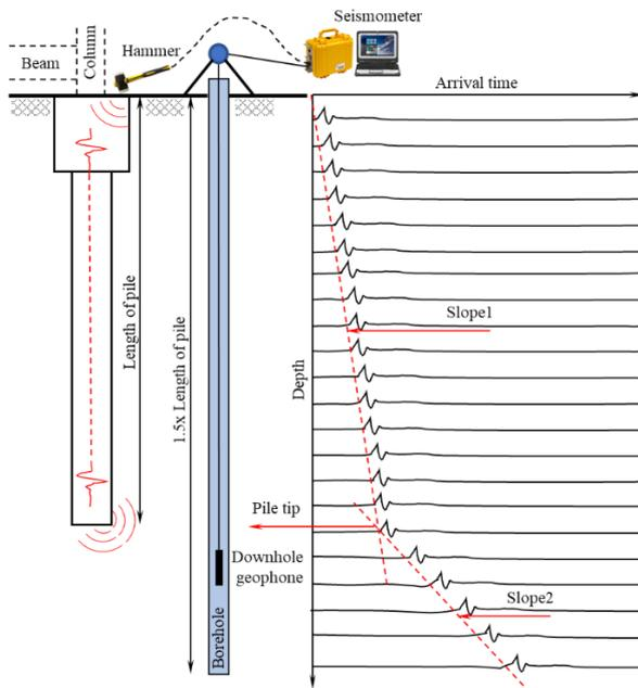
Fig. 1 Sketch of parallel seismic pile test (PSPT)
