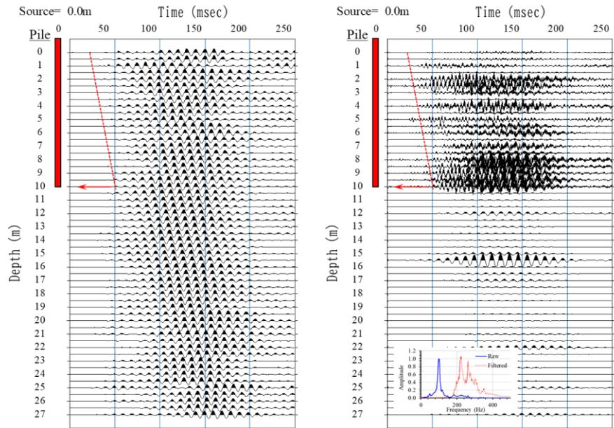
Fig. 6 PSPT result of building No.2: raw data (left) and filtered data (right)
