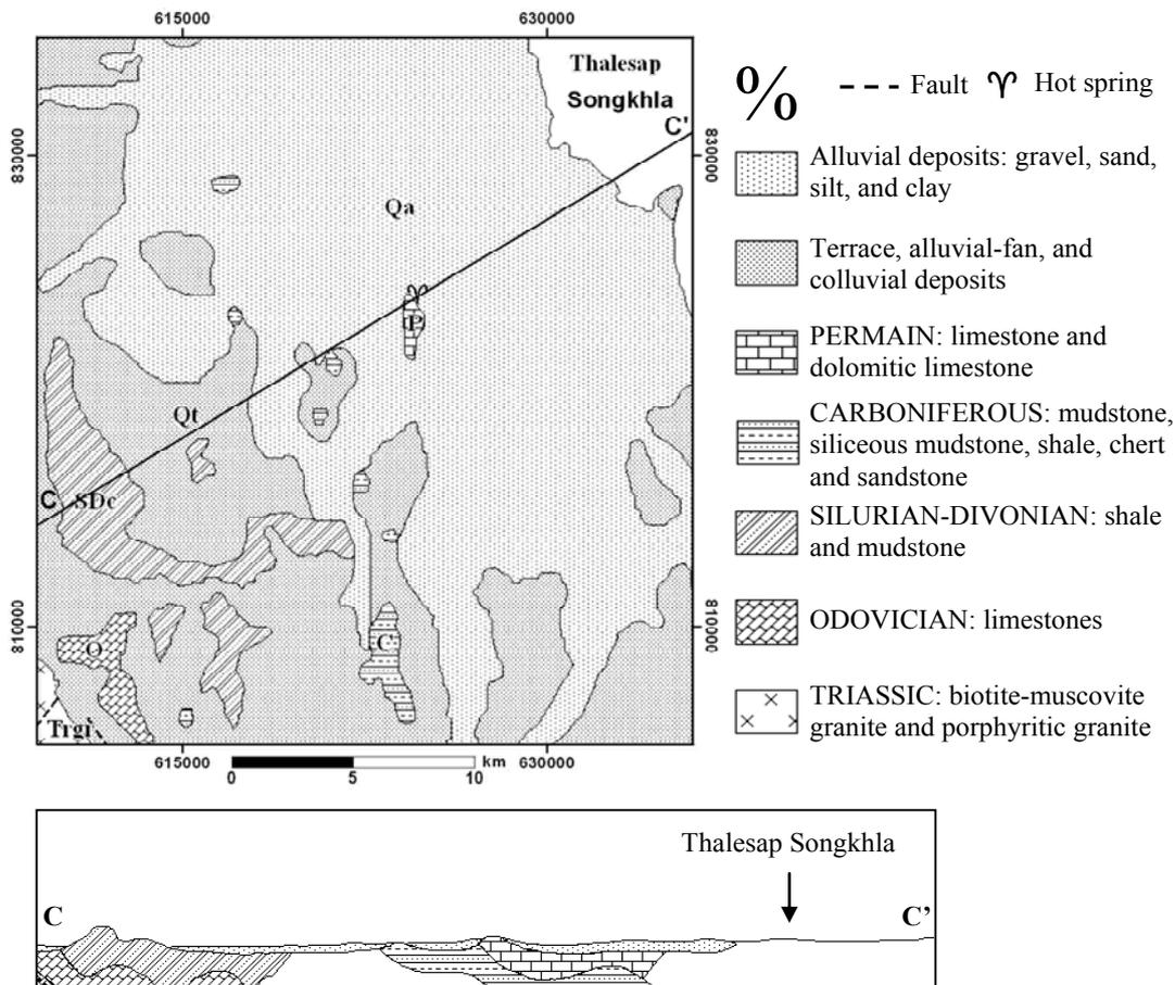
**Figure 1.** Geological map and cross section of the study area
