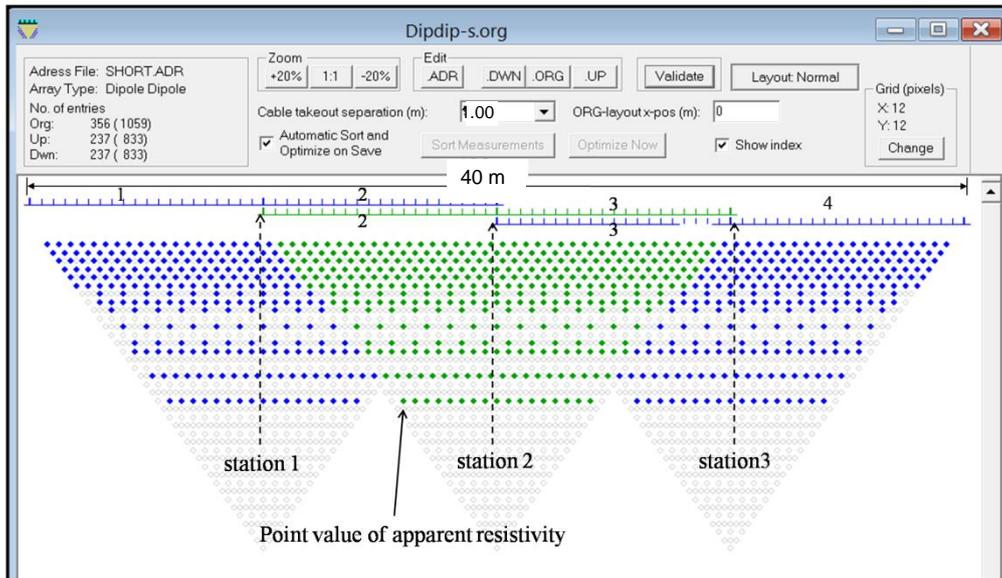
**Fig. 5.** Short protocol for dipole-dipole array resistivity measurement. Starting measurement with 2 spreads of electrodes (2 and 3), the measured apparent resistivity was then plotted in green points color. For an extension of resistivity data beneath the profiles (blue points color) the upward or downward spread needs to be performed.
