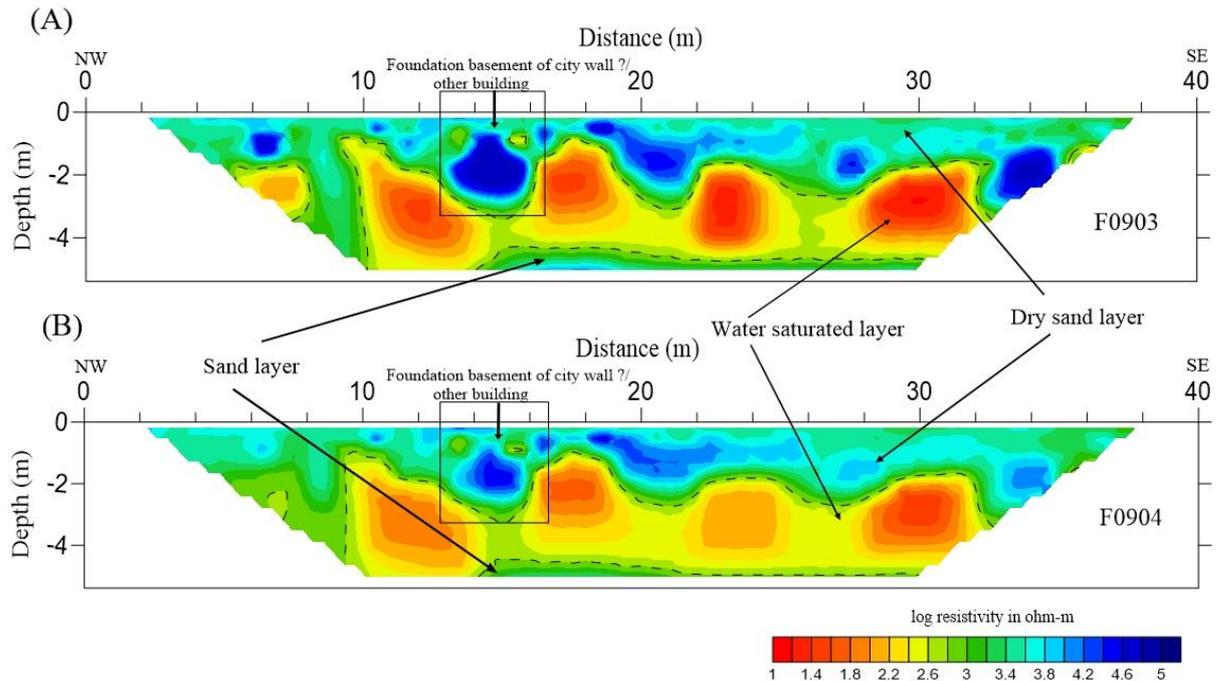
**Fig. 7.** Showing the inversion models of ERT dipole-dipole resistivity section in survey area F9, A) line F0903 and B) line F0904.
