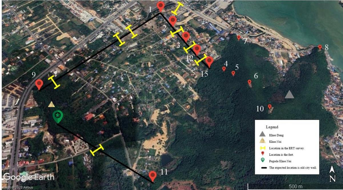
**Fig. 3.** Locations of ERT survey area (six zones) overlay on the Google Earth map. The yellow lines represent the two parallel survey lines in each zone. Only the zone 9, there are 6 survey lines.
