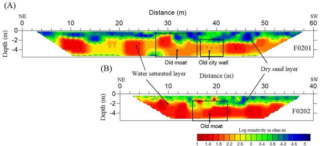
**Fig. 8.** Showing the inversion models of ERT dipole-dipole resistivity section in survey area F2, A) line F0201 and B) line F0202.
