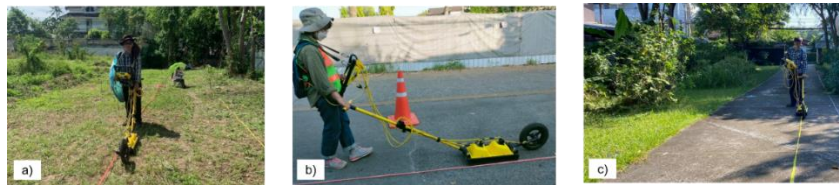
Fig. 3 GPR data acquisition using 500-MHz PulseEkko ® system on (a) vegetation soil surface, (b) concrete surface, and (c) both of surfaces.
